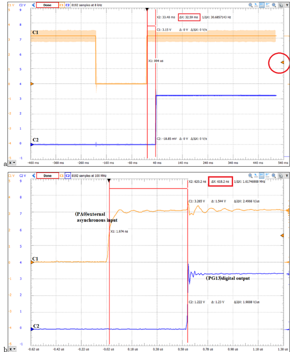
Figure 9 (A) STM32F429ZIT Cortex-M4 MCU, WaveForms software and ANALOG2 DISCOVERY DIGILENT oscilloscope to measure response time for program data transfer (32.59 ms); (B) SoC design timing report based on Xilinx FPGA and Vivado DS.
