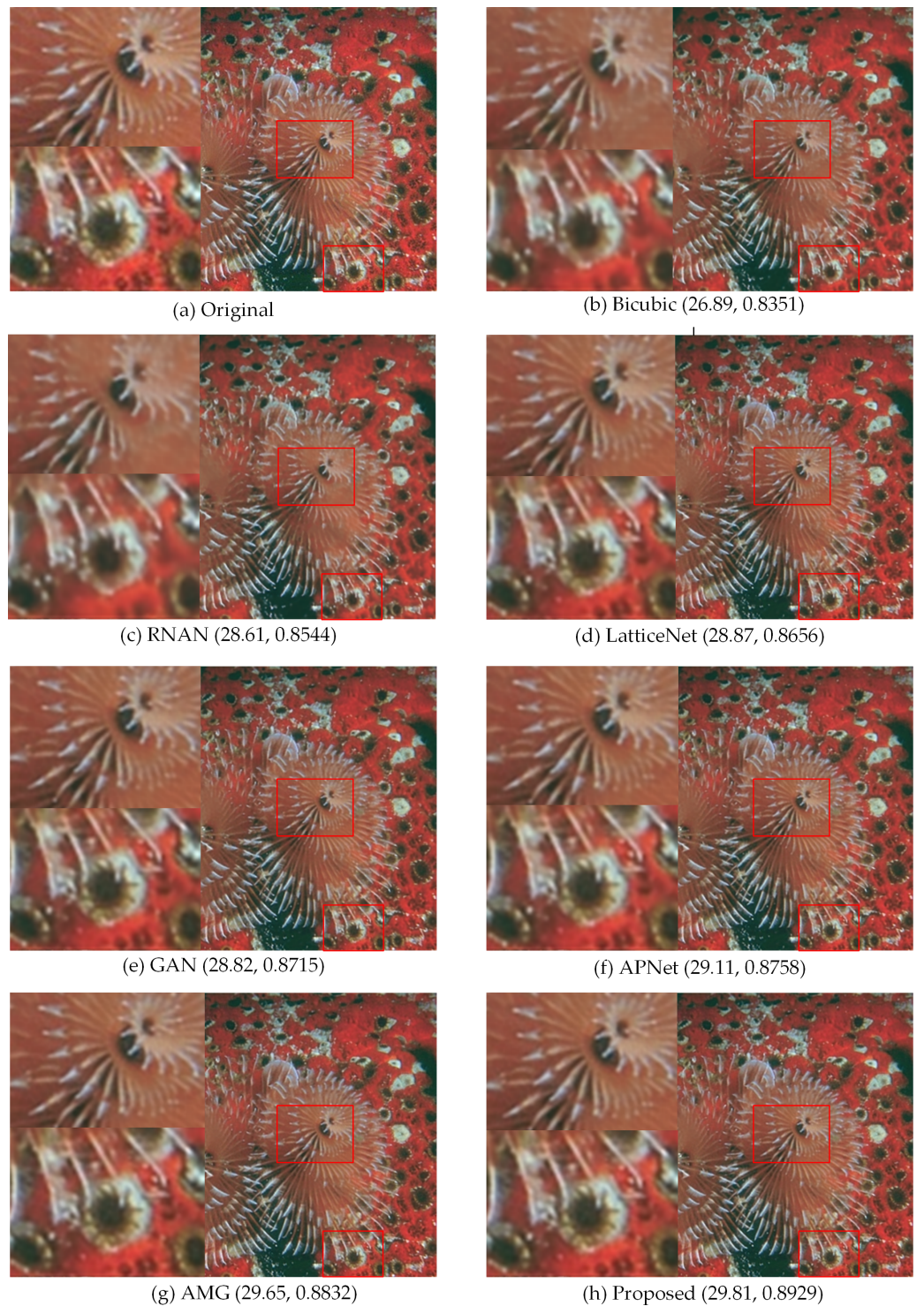
Figure 5 Compared in BSD100. The visual effects produced by different methods of 4 \times super-resolution reconstruction are compared in BSD100. Image credit: ©2001 IEEE. Reprinted, with permission, from Martin et al. (2001) .
