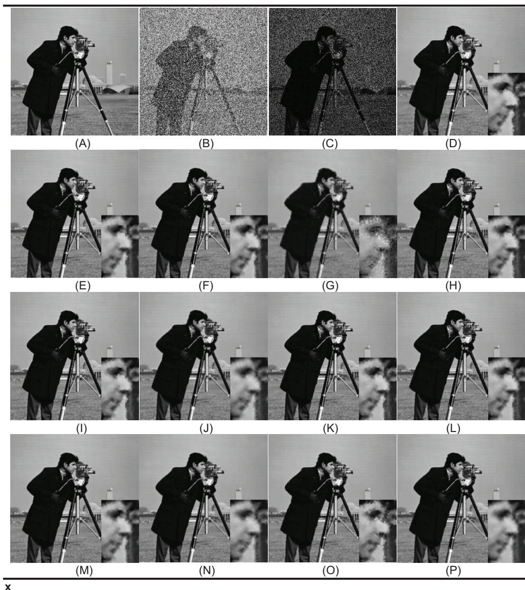
Figure 3 Denoising results by different filters for the Cameraman with the size of 512 \times 512 pixels with 60% SPN levels. (A) Original image, (B) noise of 60% (SPN) PSNR = 7.31 SSIM = 0.0204, (C) noise of 60% (PN) PSNR = 7.82 SSIM = 0.1107, (D) denoising AFMF PSNR = 30.10 SSIM = 0.9393, (E) denoising ARmF PSNR = 32.62 SSIM = 0.9630, (F) denoising IAWMF PSNR = 32.88 SSIM = 0.9646, (G) denoising ASWMF PSNR = 26.63 SSIM = 0.8406, (H) denoising AWMF PSNR = 32.12 SSIM = 0.9580, (I) denoising DAMF PSNR = 31.40 SSIM = 0.9541, (J) denoising IMF PSNR = 32.46 SSIM = 0.9558, (K) denoising TSF PSNR = 31.38 SSIM = 0.9540, (L) denoising MSCF-1 PSNR = 32.35 SSIM = 0.9606, (M) denoising DAMRmF PSNR = 32.86 SSIM = 0.9634, (N) denoising SFT_lp PSNR = 32.49 SSIM = 0.9563, (O) denoising Bilal's method PSNR = 28.74 SSIM = 0.9193, (P) denoising NVBMF (proposed) PSNR = 33.36 SSIM = 0.9630. Image source: CC BY NC; https://hdl.handle.net/1721.3/195767 . Full-size DOI: 10.7717/peerj-cs.1160/fig-3
