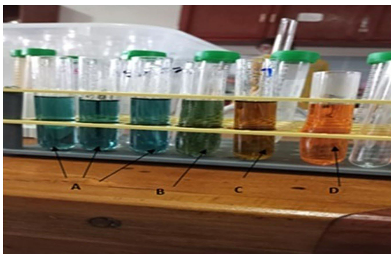
Figure 1 Methanol, ethanol and spiked methanol in acid dichromate reagent with color differences. (A) Methanol (99.8%) in acid dichromate, (B) ethanol (99.6%) in acid dichromate, (C) spiked methanol and ethanol (1:2% \text{mV}^{-1} ) in DO, with acid dichromate and, (D) reagent blank in acid dichromate.
