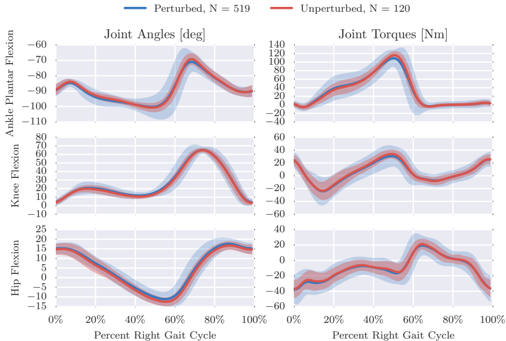
Figure 4. Right leg mean and 3\sigma (shaded) joint angles and torques from both unperturbed (red) and perturbed (blue) gait cycles from trial 20. Produced by src/unperturbed_perturbed_comparison.py .
