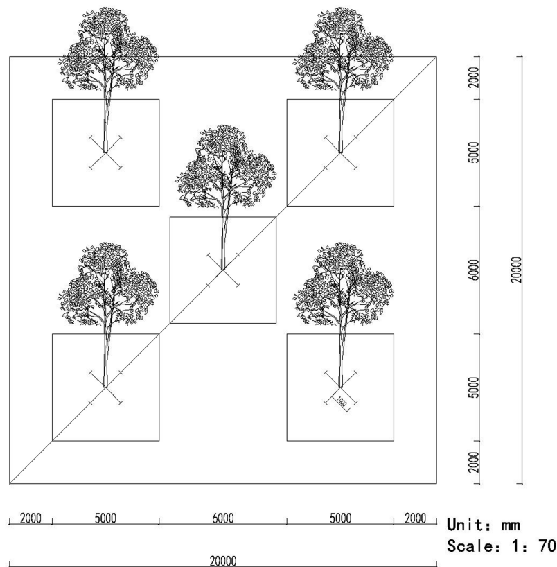
Figure 1 The pattern of the five-point method for sampling the roots and soils.
