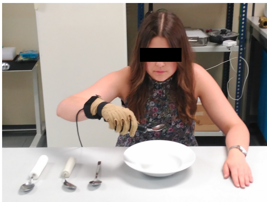
Figure 2 Subject wearing the instrumented glove performing the task of eating with a spoon.
