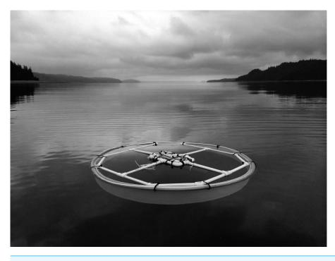
Figure 2 Neutrally buoyant Lagrangian drifter (diameter 0.8 m), with GPS unit at center. Photo credit: Micah Horwith
