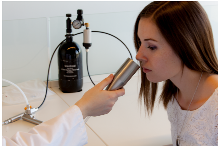
Figure 3 Olfactory threshold testing using the Scentroid SM110C olfactometer and SK5 n-butanol Sensitivity Kit.
