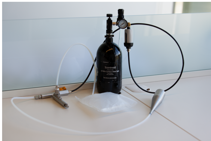
Figure 1 Scentroid SM110C olfactometer used in measuring n-butanol olfactory thresholds.
