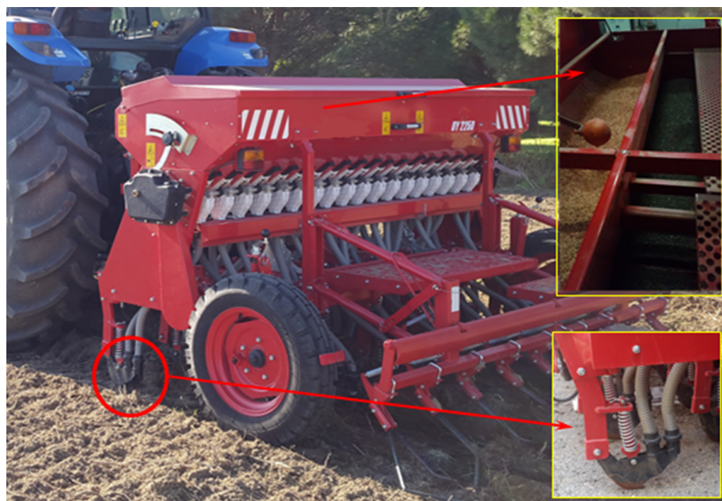
Figure 1 Combined seed drill and mixed seeding condition.
