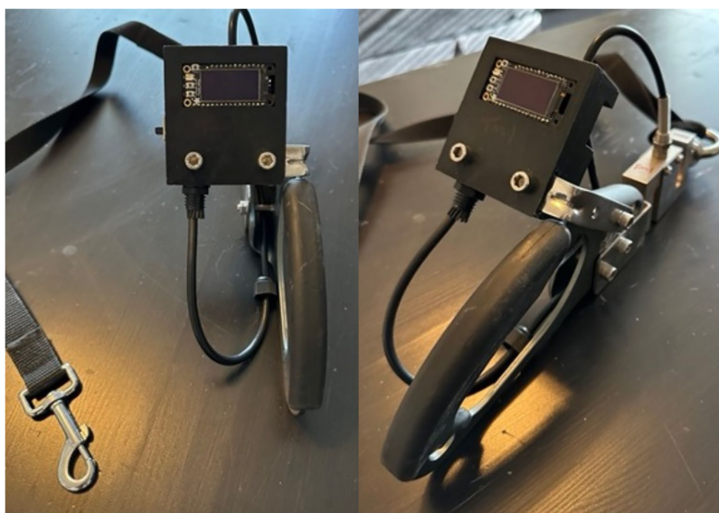
Figure 2 Strain gauge. The panel on the left depicts the computer attached to the ascender handle held by handler. The panel on the right depicts eye-bolt attachment connected to the load-cell sensor on one end and leash on the other. Source: own photo.
