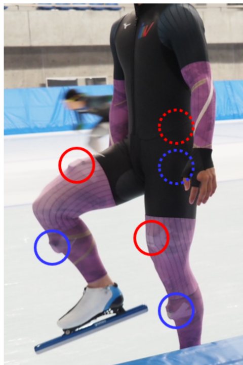
Figure 1 IMU sensors attached to a speed skater. Red dotted circle, lower thoracic. Blue dotted circle, Pelvis. Red circle, Thigh. Blue circle, Shank. UT and Pel are affixed to the back and cannot be seen directly.
