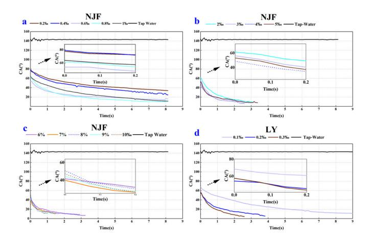
NJF droplets spread on wheat leaf adaxial surface during the observing time.
