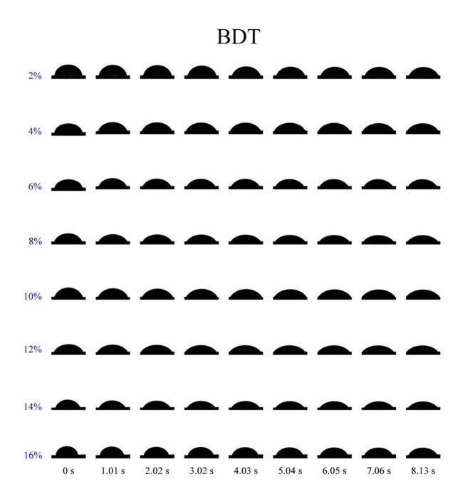
VP droplets spread on wheat leaf adaxial surface during the observing time.
