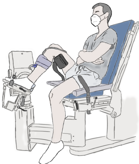
Figure 1 Illustration of the experimental setup. A dorsiflexion attachment over the metatarsals limited ankle joint rotation and force contributions from the toe extensors to the measured net ankle joint torque during maximal voluntary fixed-end dorsiflexion contractions. A cushioned support was fixed underneath the distal right femur to support the right thigh. A 6 cm flat linear-array ultrasound transducer was located underneath the self-adhesive strap around the right mid-shank to image the tibialis anterior (TA) muscle with B-mode ultrasound. The two surface electrodes immediately distal to the transducer recorded the single differential myoelectric signal over the TA via surface electromyography. Participants were instructed to fold their arms across their stomach and to focus on pulling the top of their foot towards their shank using only their dorsiflexor muscles.
