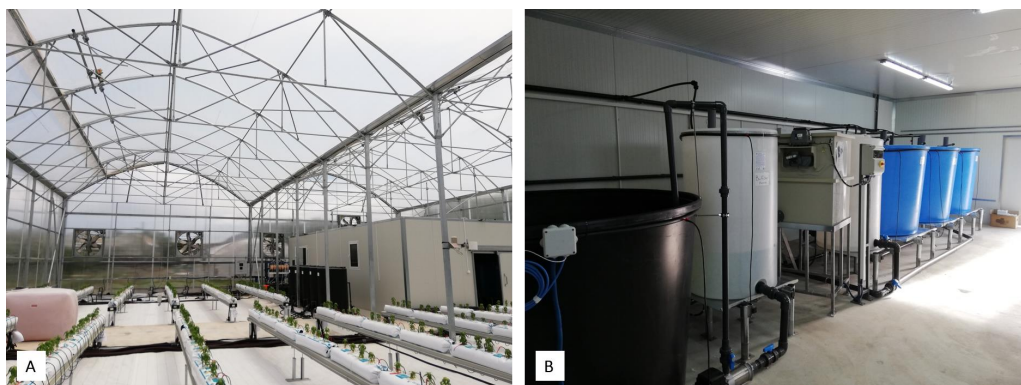
Figure 1 The aquaponics unit. Plant cultivation area (A) and RAS chamber (B) of the pilot-scale aquaponics greenhouse at the first days of the experiment.
