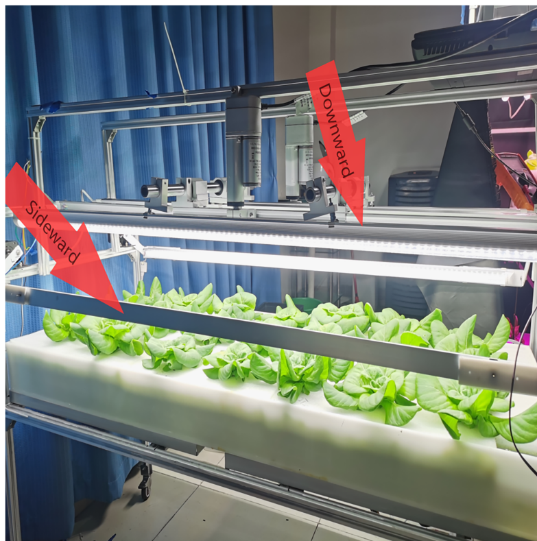
Figure 5 The combination of the movable downward lighting and supplemental adjustable sideward LED lighting.
