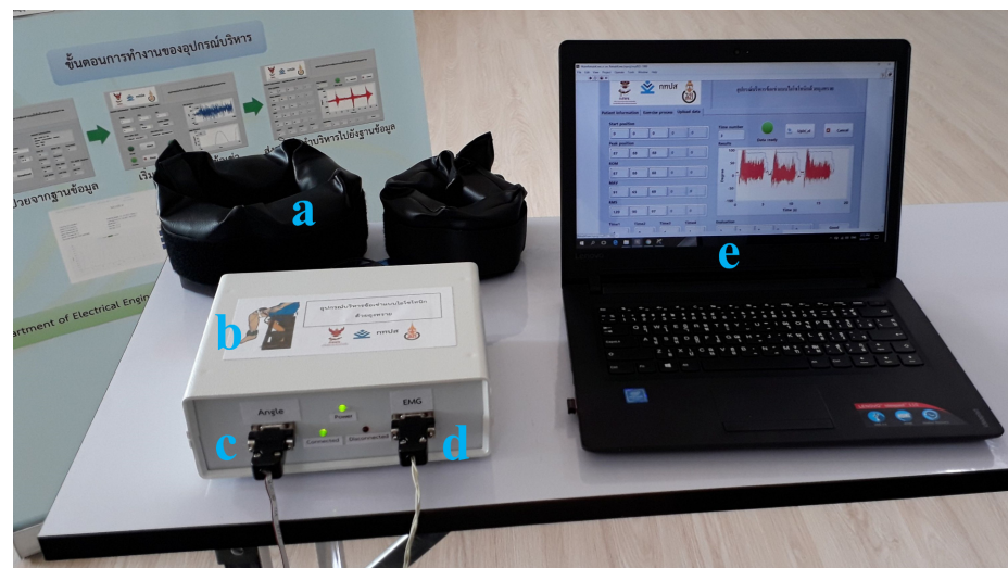
Figure 1. Isotonic exercise monitoring device and its peripheral equipment: (a) sandbag, (b) isotonic exercise monitoring device, (c) triaxial accelerometer channel for knee angle measurement, (d) sEMG channel, (e) graphic user interface (GUI).
