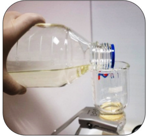
(c) Membrane filtration
