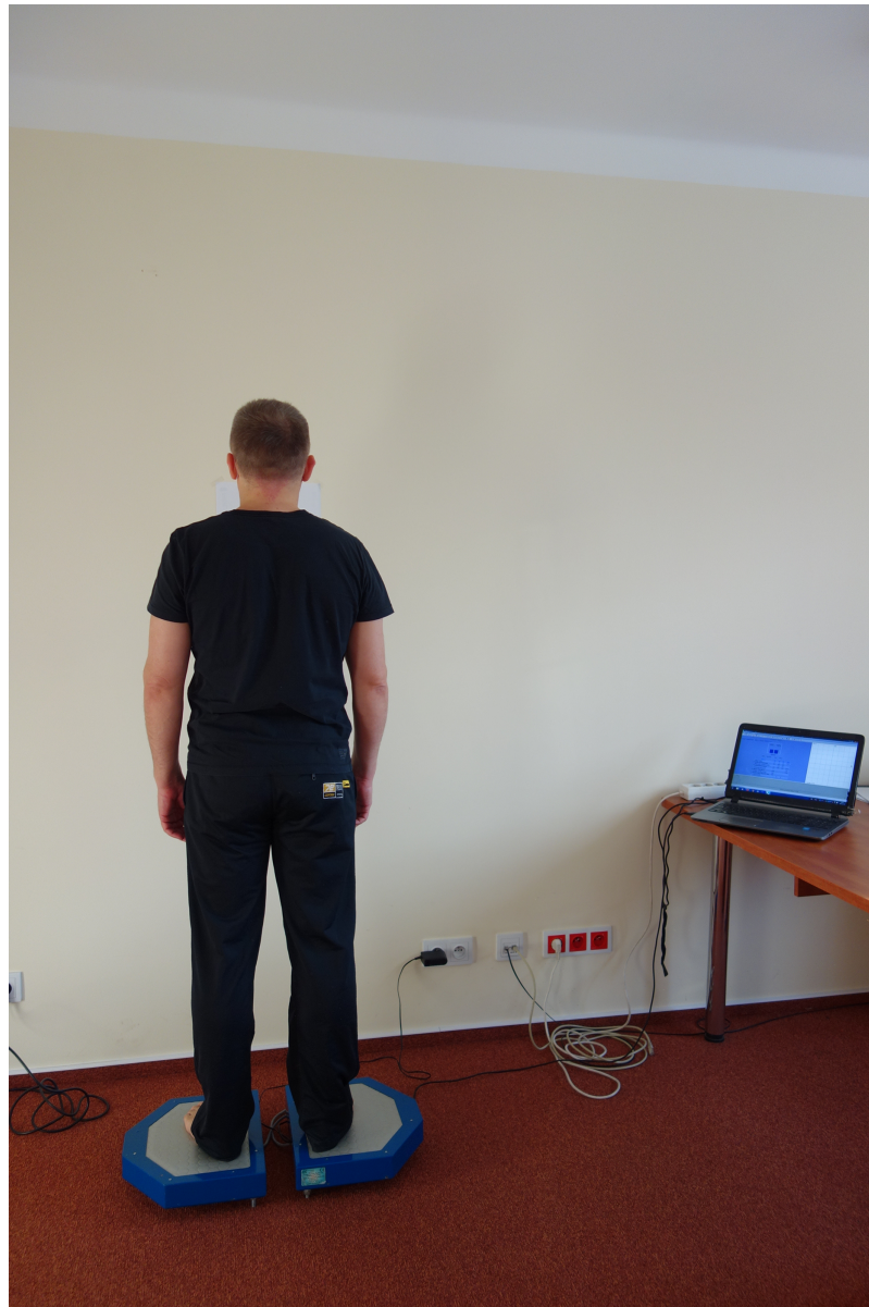
Figure 2 Presentation of measurement equipment- bi-modular stabilometric platform CQStab2P.
