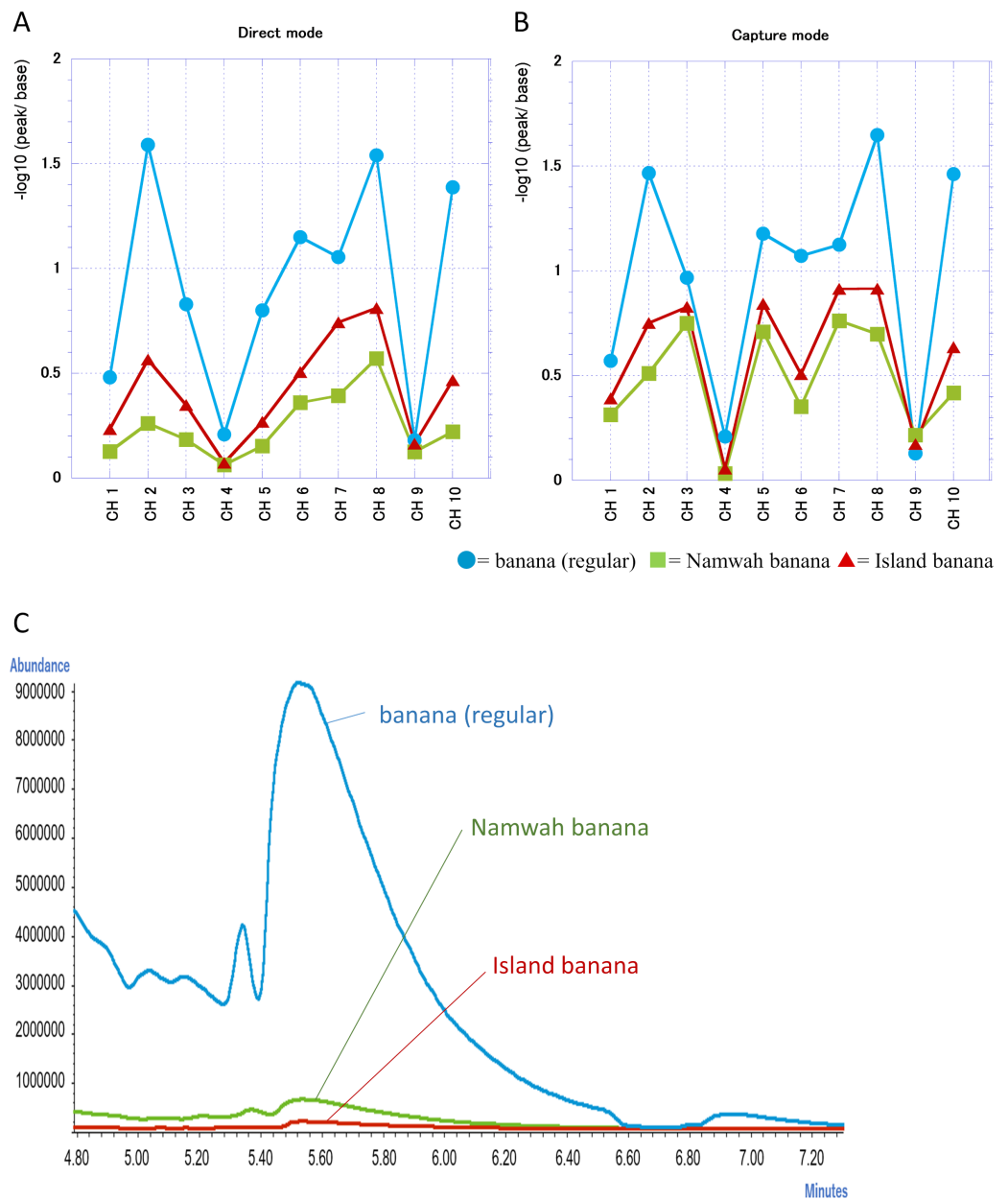
Figure 9 Comparison of shop S regular bananas with Island banana and Namwah banana juice. (A–B) Change of the resistant value in each channel of FF-2A. (A) Direct mode, (B) Capture mode. (C) Chromatogram comparison.
