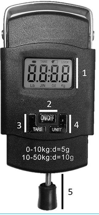
Figure 1Adapted pressure algometer—PA. (1) Display; (2) On-Off button; (3) Tare button; (4) Unit<br/>selection button; (5) Adapted terminal.Full-size im DOI: 10.7717/peerj.10162/fig-1
