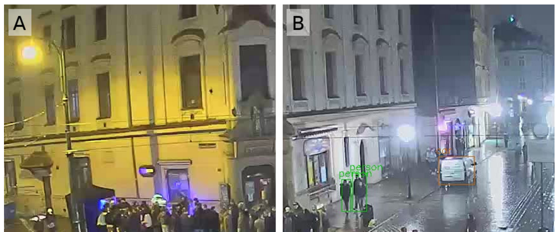
Figure 3. The upper left two tiles from the split image (Fig. 2). Pedestrians (A) undetected and (B) detected by YOLO tiled method.
