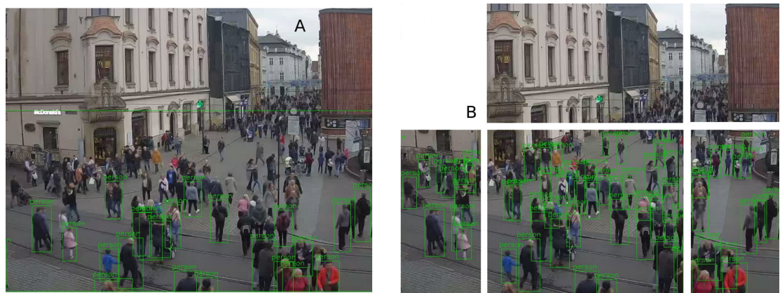
Figure 4. Pedestrian detection from All Saints Square webcam by (A) YOLO and (B) YOLO tiled method. Both views are framed to the central part. YOLO tiled view without the upper left tile.
