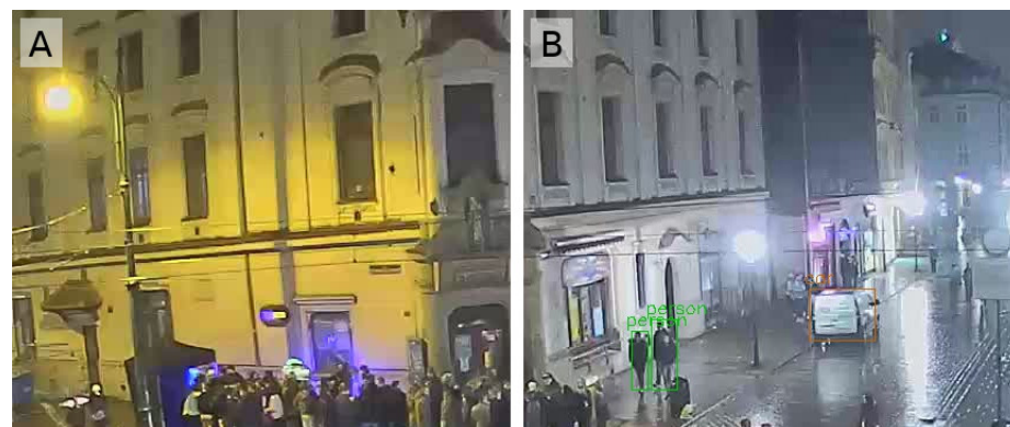
Figure 3. The upper left two tiles from the split image (Fig. 2). Pedestrians (A) undetected and (B) detected by YOLO tilde method.
