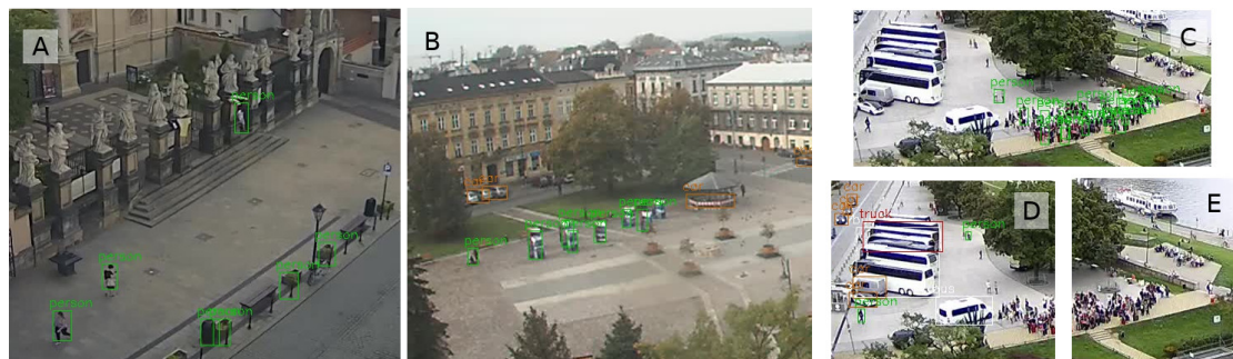
Figure 8. The biggest difference in pedestrian detection for three webcams – less pedestrians from YOLO tilde method. Error assigning class: (A) trashcan from Grodzka (bottom right), (B) advertisement display from Podgorze (only one real person was detected). Better detection of people in crowd from Wawel webcam (C) by YOLO compared to (D)(E) YOLO tilde method.
